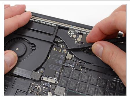
Use the tip of a spudger to pry the three AirPort antenna cables straight up off of their sockets on the AirPort board.
